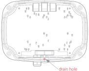
\*Data package containing Base Plate Hole Dimensions drawing and maximum inner clearance height can be found in Download list \*\*IP66 rating can be achieved by sealing the drain hole
