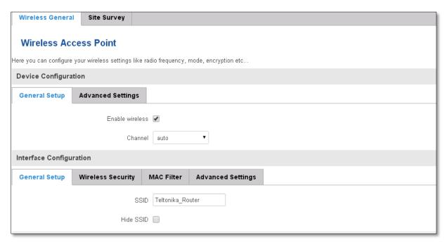
Here you can see the Overview of the wireless configuration. It is divided into two main sections – device and interface. One is dedicated to configuring hardware parameters other – software.
