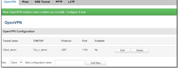
To see at specific configuration settings press "edit" button located in newly created configuration entry. A new page with detailed configuration appears, as shown in the picture below (TLS client example).
