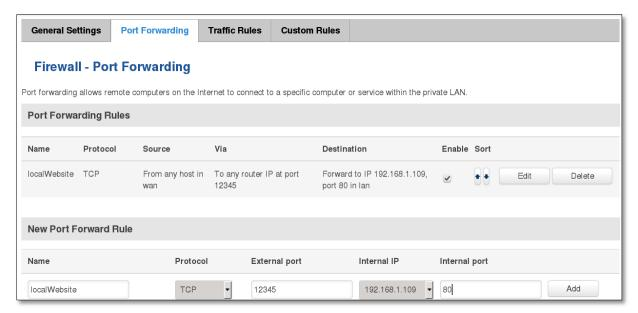
You can use port forwarding to set up servers and services on local LAN machines. The above picture shows how you can set up a rule that would allow a website that is being hosted on 192.168.1.109, to be reached from the outside by entering http://routersExternallp:12345/.
