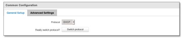
You can switch between the Static, DHCP or PPPoE protocol by selecting the protocol that you want to use and then pressing **Switch Protocol**
