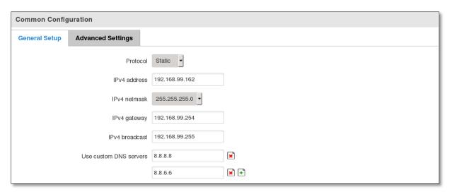
This is the configuration setup for when you select the static protocol.
