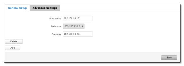
As you can see, the configuration is very similar to the static protocol; only in the example a 99th subnet is defined. Now if some device has an IP in the 99 subnet (192.168.99.xxx) and the subnets gateway metric is "higher" and the device is trying to reach the internet it will reroute it's traffic not to the gateway that is defined in common configurations but through the one that is specified in IP aliases.
