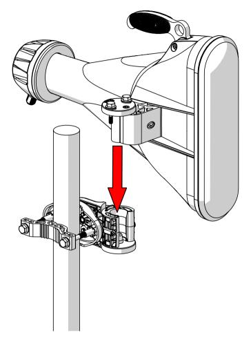
Model HG3-CC-A60 shown. Installation instructions are identical for other Asymmetrical Horn models. Antenna dimensions may differ.
