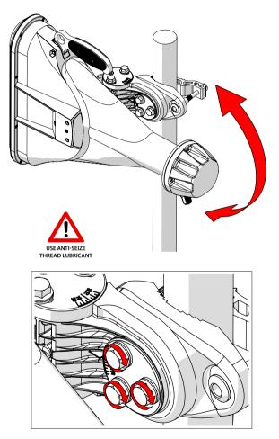
Model HG3-CC-A60 shown. Installation instructions are identical for other Asymmetrical Horn models. Antenna dimensions may differ.
