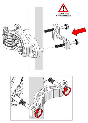
Model HG3-CC-A60 shown. Installation instructions are identical for other Asymmetrical Horn models. Antenna dimensions may differ.
