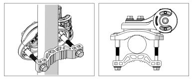
Place the AH-CC bracket as shown below for the span of pole diameters 50 - 80mm.
